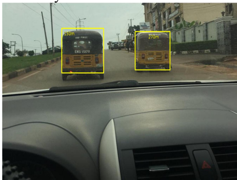
Fig. 15: Results of System Integration with Two Vehicles
