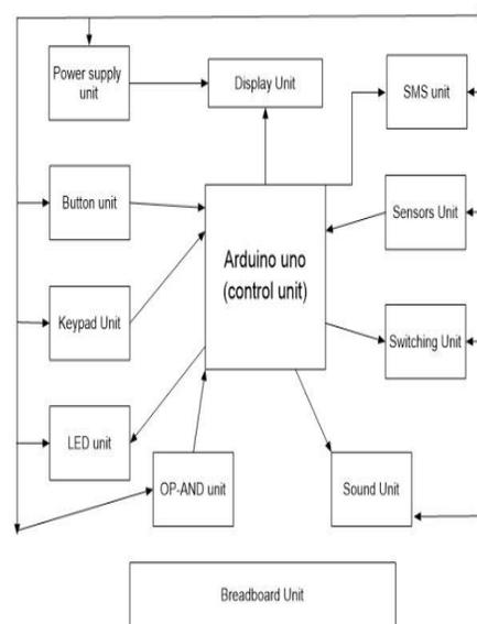
Figure 6: Block Diagram of Arduino Experimental Training Kit
