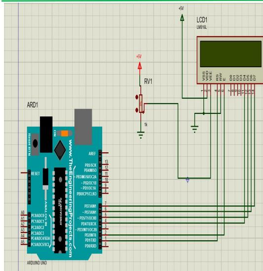
Figure 11: LCD Interfaced to Arduino Uno
