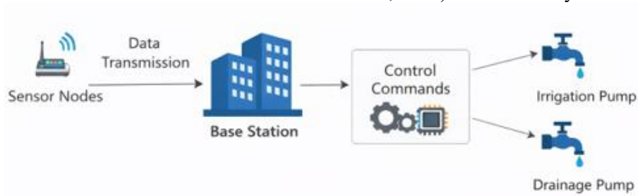
Figure 2: Data Flow Diagram Showing Sensor Data Transmission and Control Commands
