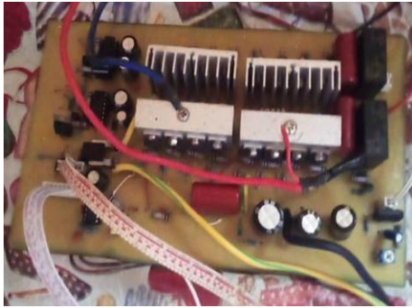
Figure 6: Inverting Unit Circuit Board with Changeover and Filter Circuit
